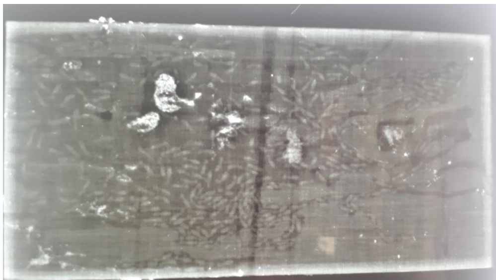
Image 3. X- Ray image of Heterotermes inside plywood.
